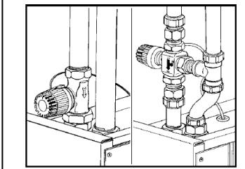
3. Remove grommet and feed sensor bulb through top of casing.
